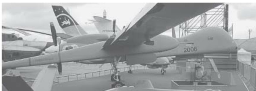
The Israeli drone Heron TP can stay in the air for up to thirty-six hours, fly at a maximum speed of 230 miles per hour, and carry more than a ton of cameras and bombs.
